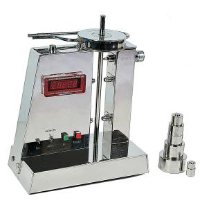
Instrument used to measure the viscosity of range of fluids from liquid to viscous materials. A sturdy instrument suitable for day to day industrial usage.
