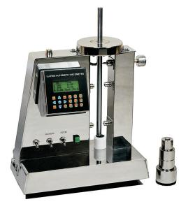
Lloyds has designed a 2nd generation of Laray Viscometer for instant and in-depth analysis of your viscosity measurements. An Instrument that uses the advance automation tools to directly calculate the Viscosity and other related parameters eliminating the cumbersome traditional time consuming calculation on graph sheet or computer software. A sturdy design which can withstand day to day industrial usage.
