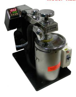
Lloyds Laboratory Rub Resistance Tester is a tool for comparing the rubbing, scuffing and marking of inks and coatings on commercial print and packaging, it can be used as part of quality control in a production environment or an aid to development in the laboratory.
